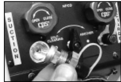
**BUILT-IN 100 MESH PARTICLE FILTER**
