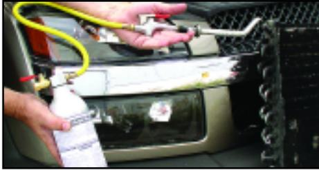
Reduce comebacks by flushing evaporator & condenser with the **TLFG**. Simply add solvent and use shop air to reverse flush the component. **TLFGXT** - Replacement tip for flush gun.
