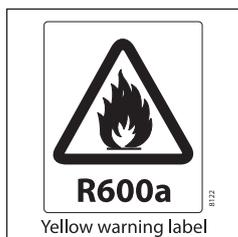
R600a is flammable in concentrations of air between approximately 1.5% and 8.5% by volume (LEL lower explosion limit and UEL upper explosion limit). An ignition source at a temperature higher than 460°C is needed for a combustion to occur.
