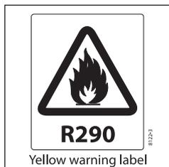
R290 is flammable in concentrations of air between approximately 2.1% and 9.5% by volume (LEL lower explosion limit and UEL upper explosion limit). An ignition source at a temperature higher than 470°C is needed for a combustion to occur.
